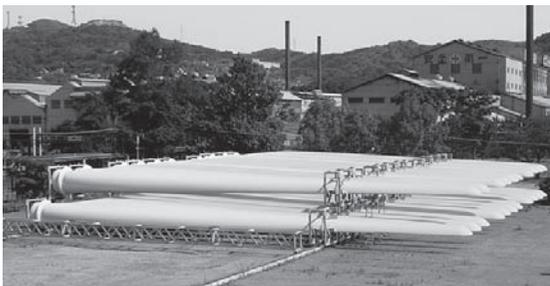
Fig. 3 Blades for wind turbine
