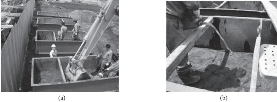
Fig. 5 Construction of experimental tabs (a), and artificial pollution of soils with petroleum (b).
