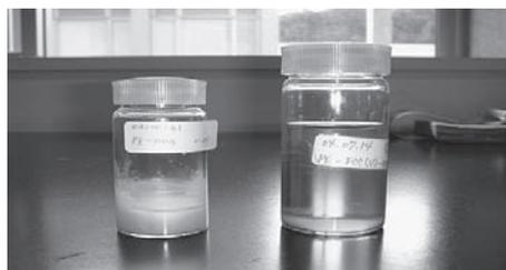
Fig.5 Cracked oils of PE (L : Non catalytic, R : Catalytic)
