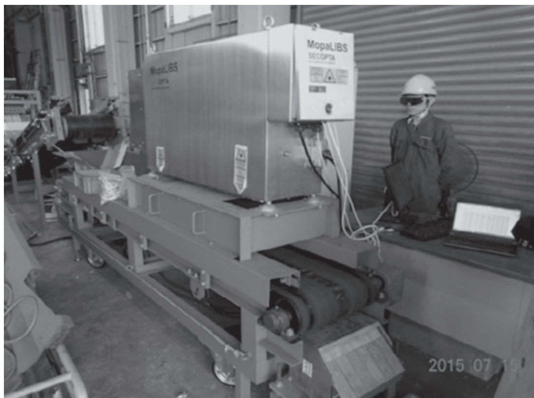
Fig.6 The first LIBS sorter developed in the world.
