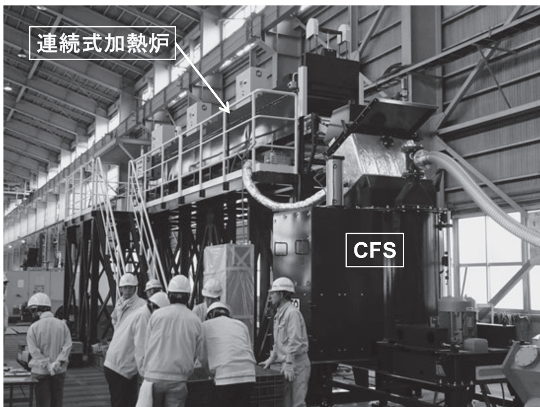
Fig.2 Pilot plant of cross flow shredder with heating furnace for detaching devices for printed circuit board.
