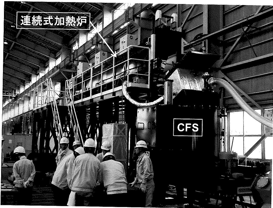
**Fig.2** Pilot plant of cross flow shredder with heating furnace for detaching devices for printed circuit board.
