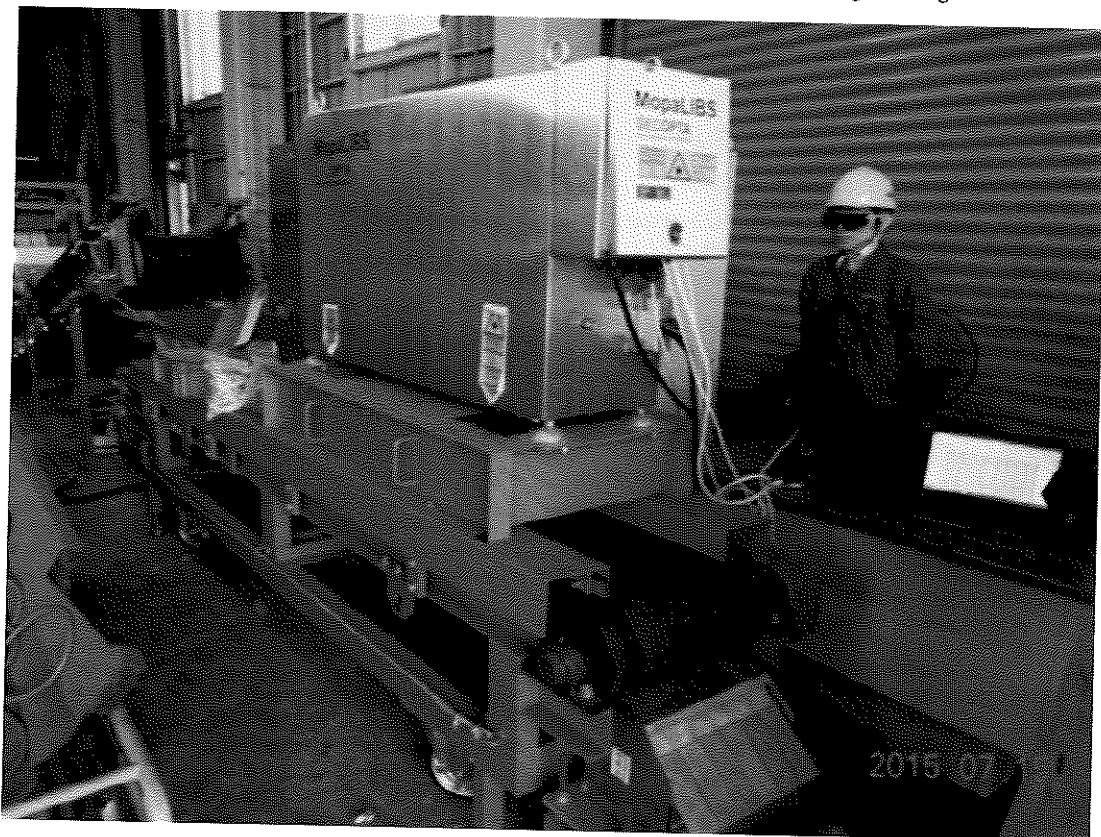
Fig.6 The first LIBS sorter developed in the world.
